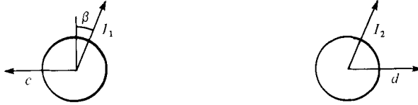
FIGURE 2. The devices, the incident wave represented by I_1 and I_2 , and the interaction effects represented by c and d .
